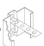
**MASONRY "T"-SHAPED:** A loose metal device used to secure the frame to new masonry walls.
