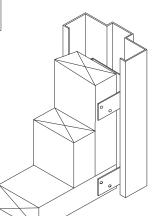
**WOOD STUD:** A metal device secured in a frame to be used for attachment in a wall built with wood studs.
