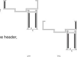
**REGULAR ARM:** Reinforcing in pull side face of frame header, transom mullion, or panel.
