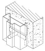
**FIXED FLOOR:** A metal device attached to the bottom of the frame to secure a frame to the floor. Also referred to as Base Anchor or Sill Anchor.
