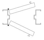
**COMPOSITE DOOR:** A door consisting of a nonmetal core bonded to a metal facing.
