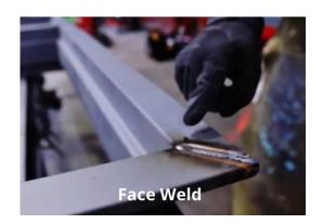
Some specifications only state "welded frames" and not whether they want face welds or full profile welds. In instances like this where **full profile welds** are not requested, specifiers can expect to receive **face welded** frames.
